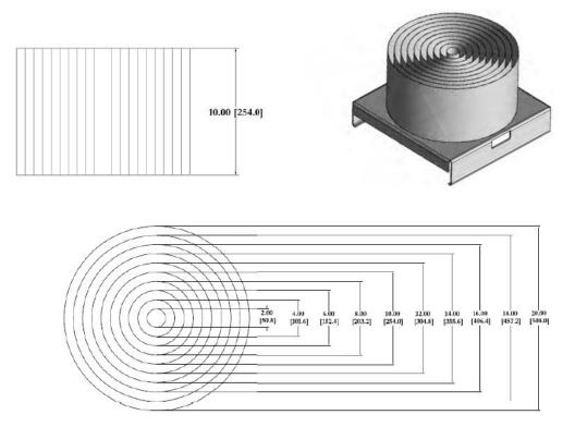
Figure 2.4: Annular Ring Specifications
