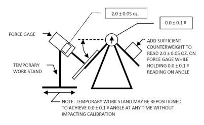
Figure 2.3: Force Balance Calibration Procedure
