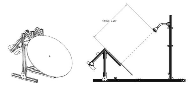
**Figure 1 Force Balance Test Apparatus**
