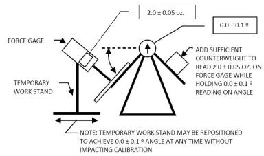
Figure 3 Force Balance Calibration Procedure
