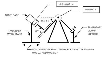
**Figure 2 Force Balance Calibration Setup**
